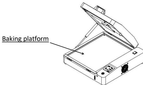
**4.1.** Open the baking lid, place the image to be baked (powder side up) on the baking platform for baking and color fixation. After baking is completed, open the baking lid, take out the image on the baking platform, and baking is complete.
