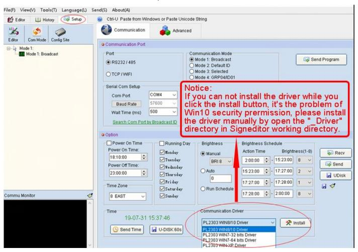
After Install the communication driver ready, Connect the led display with computer, Set the communication port in RS232/RS485(USB/RS232/RS485 communication), Communication mode choose Mode 1: Broadcast. Click "Search Com Port by Broadcast ID" then will find the com port.
