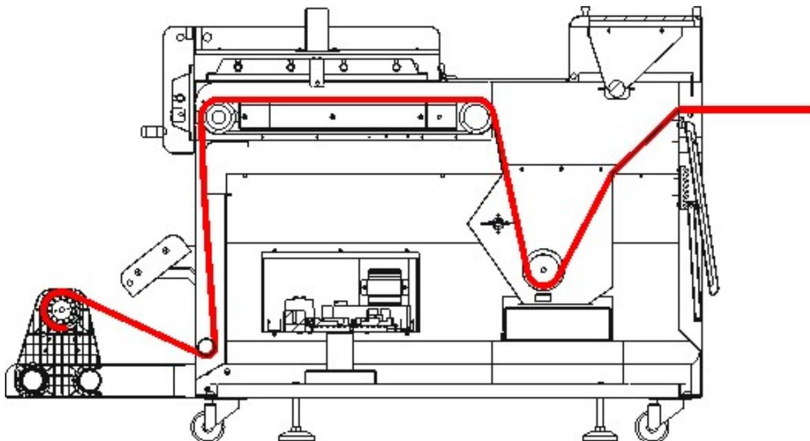
**2.1** Lead the media into powder box, though outside powder bar, and then cross the space between up dryer and platform dryer, wind the media to the paper tube of the take up winder, the winding operation complete.
