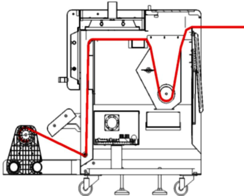
**2.1** Lead the media into powder box, though outside powder bar, and then cross the space between up dryer and platform dryer, wind the media to the paper tube of the take up winder, the winding operation complete.
