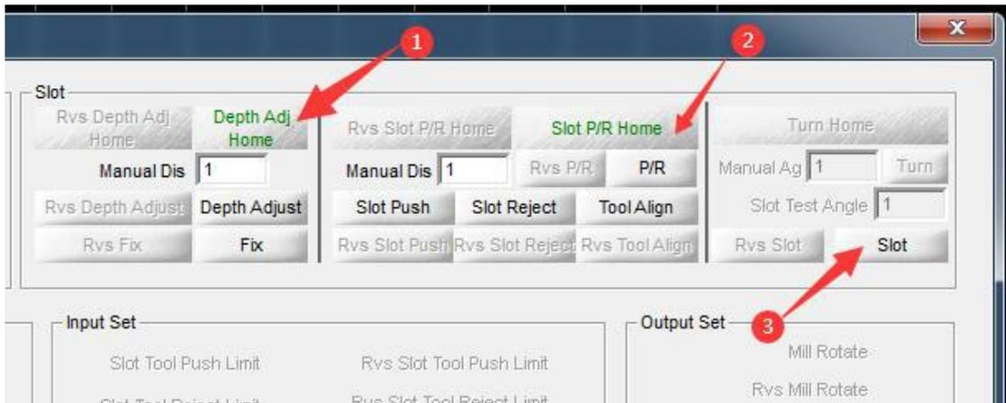
⑨ Forward--Check the depth of the slot
