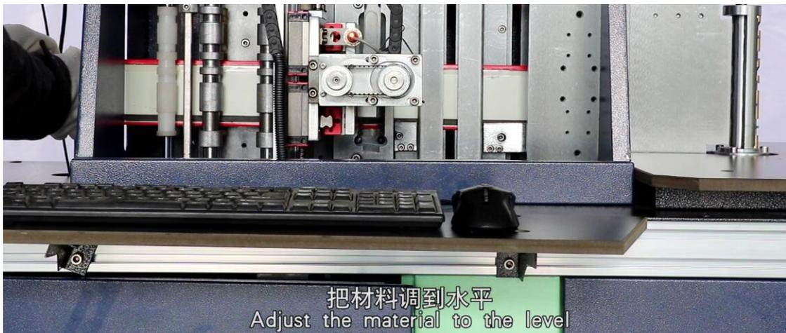
6. And we can see ,as follow picture , press the button ,the rubber wheel will loose ,and press twice , the rubber wheel will fix .when we feed the material ,we need to loose it.
