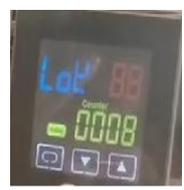
The interface displays 88, and then press the setting key
