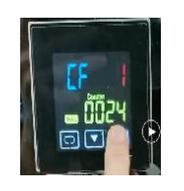
Press ▲ key once, and the screen will display as shown in the figure. At this time, it will display °F in the upper right corner of 1
