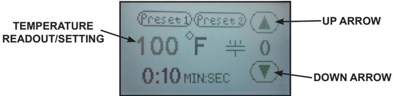
1. Touch the temperature readout on the display. “UP” ▲ and “DOWN” ▼ arrows will appear on the right side of the display and the temperature value will start flashing and to indicate it is in set mode.
