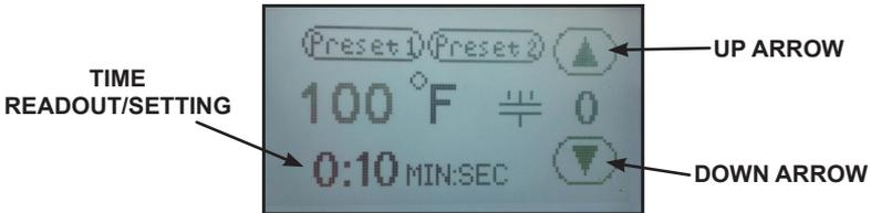
1. Touch the time readout on the display. “UP” ▲ and “DOWN” ▼ arrows will appear on the right side of the display and the cycle time value will start flashing and to indicate it is in set mode.
