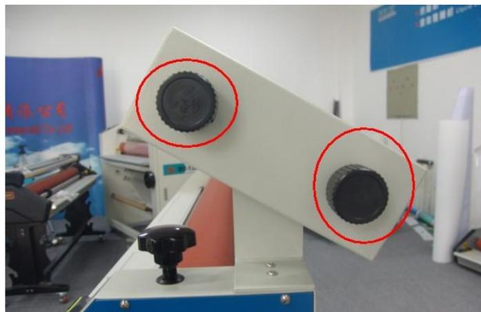
**Raising and lowering the rollers:** The rollers can be raised or lowered by turning the knobs clockwise or counter-clockwise. When turning counter-clockwise and the two rollers meet each other, the hand wheel is turned with ease at this 'space position'. Keep on turning knobs to increase the pressure of the rollers. It has been left to the operator's device to choose the proper pressure according to the material at hand. (In most cases, we recommend the 'Idler position'.)
