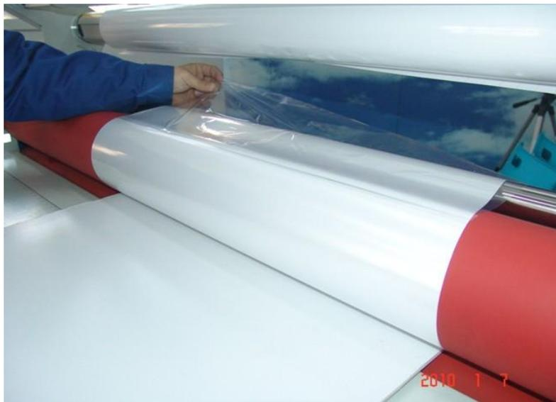
Step 5. Manully peel liner, and then press Pedal switch to run mounting.
