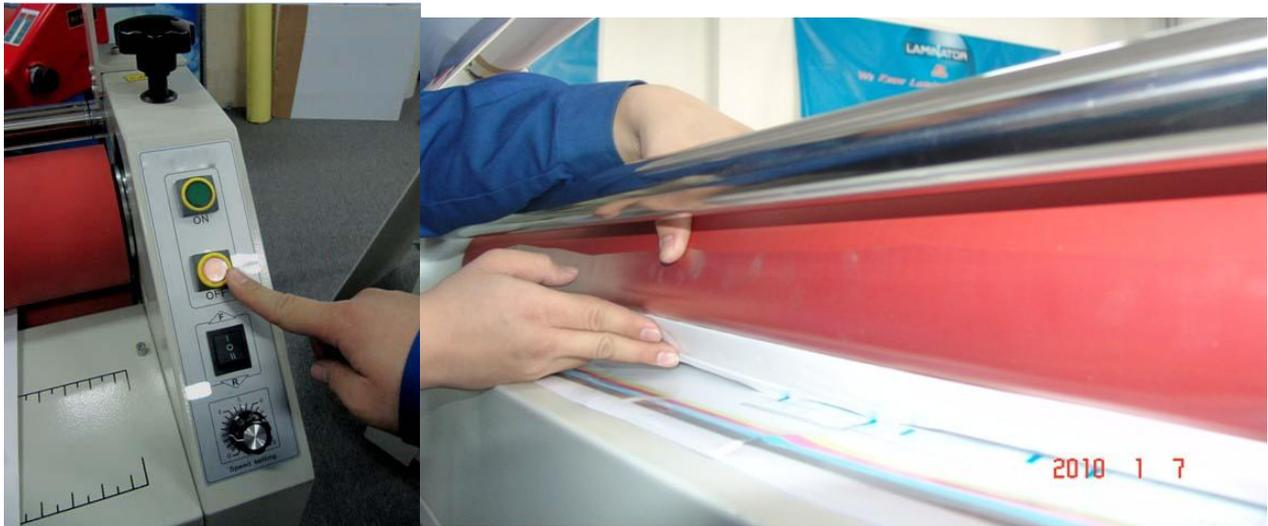
Step 3. Separate film and liner paper, fold liner around 10cm, press pedal switch to run till the prints and film ends then stop, after rotate roller a bit backwards to rear working table manually in case the prints run out of rollers.
