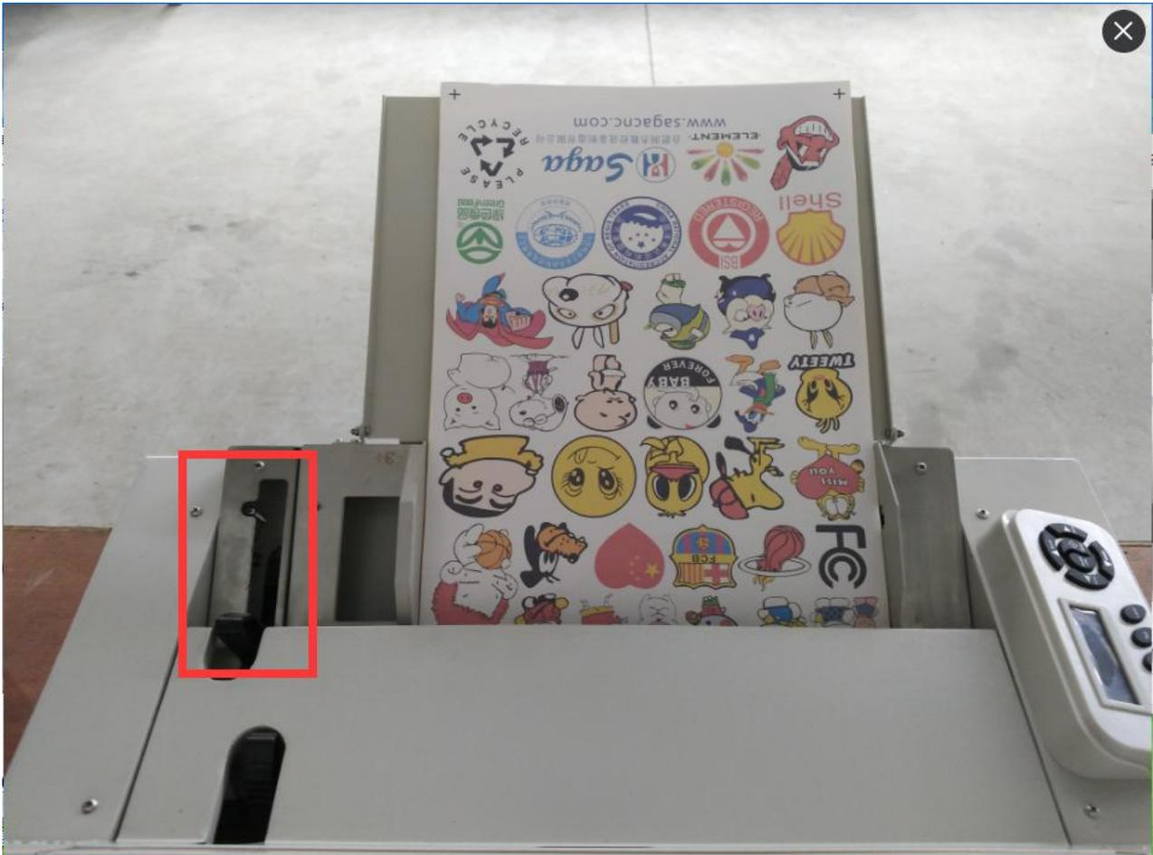
Step2: Installed blade holder (make sure the blade force is appropriate)
