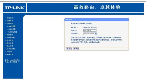
Set the router IP address as 192.168.2.1 (different with mainboard or other connected router)
