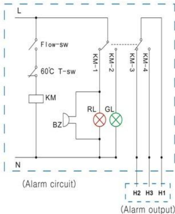
**The cooling water circulation loop alarm causes and the work of the state table**
