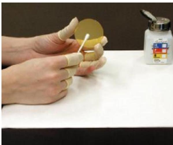
the optic against the mount to remove the polish residue. Repeat this step several times if necessary to assure that no polish residue is left on the optic's edges when the cotton swab is lifted from the surface.]
