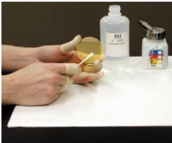
Use only high-quality surgical cotton balls that have been sorted to remove any with embedded abrasives. White distilled vinegar with a 6% acetic acid content should be used.
