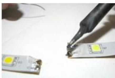
**Step #3:** Solder two pre-tinned wires onto the solder pads of the first strip. Try to stay consistent with red as (+) and black as (-). The wires should be long enough that you can hold on to them while soldering.
