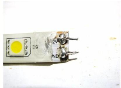
**Step #5:** With the flex strips touching each other end-to-end, match the color code letters on both strips (You may have to turn around one of the strips if they don't match up). Then, solder the wires to the end of the second strip, forming a bridge.
