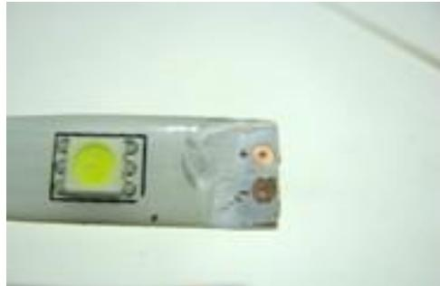
**Step #2:** With a hot, clean soldering iron, use Rosin-Cor solder to pre-tin the solder pads. It won't take long to heat the strip so be quick!
