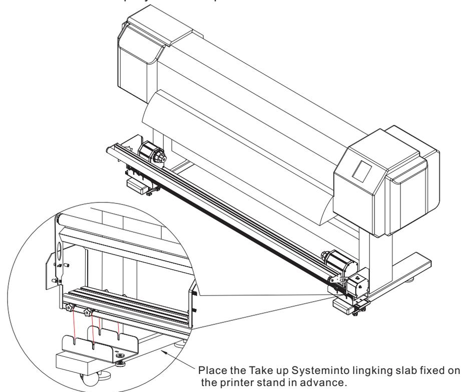
Place the Take up System into linking slab fixed on the printer stand in advance.
