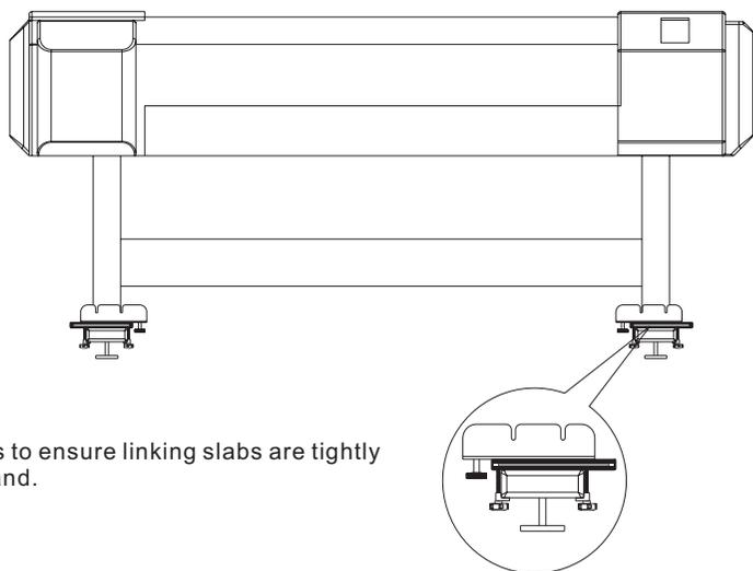
Tighten the screws to ensure linking slabs are tightly fixed on printer stand.
