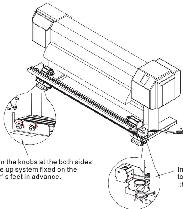
Tighten the knobs at the both sides of take up system fixed on the printer's feet in advance.
