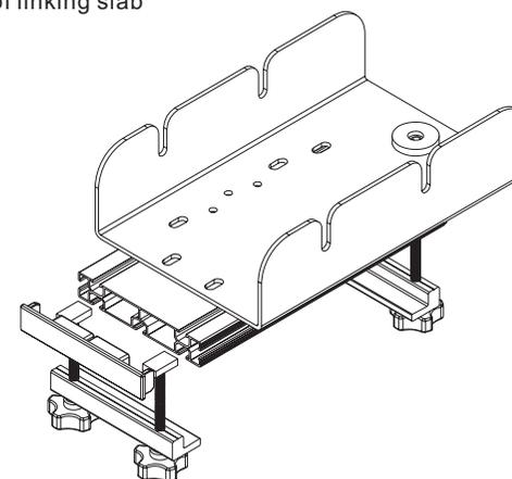
Open plastic cover and slip the fasteners into aluminum bar, then install the cover.
