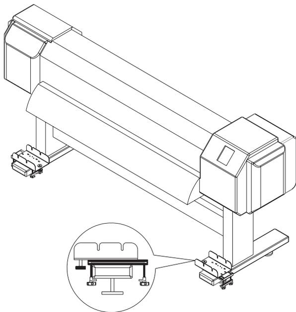
Install linking slabs to printer stand, pay attention to installation direction.
