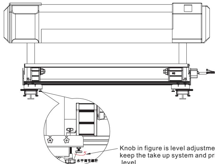
Knob in figure is level adjustment screw, used to keep the take up system and printer in the same level.
