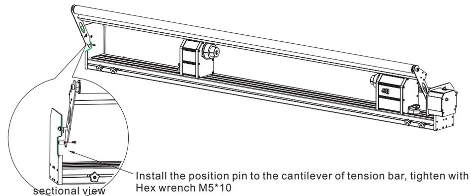
Install the position pin to the cantilever of tension bar, tighten with Hex wrench M5\*10
