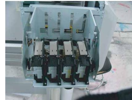
7. Remove Ink ID Cable Assy (VJ16 to J19) and I/C Cable Assy (J8 to J11) of the targeted Cartridge holder Assy from JUNCTION Board Assy.
