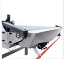
Additional aspiration kit for unloading belt consisting of 2 suction hoods, on the top and end of the belt.
