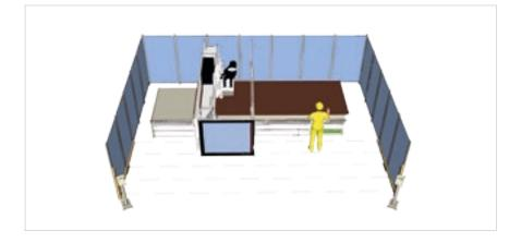
The machine can be configured with **tandem loading** in order to alternately process panels. This allows for loading or unloading to be carried out during machining operations.
