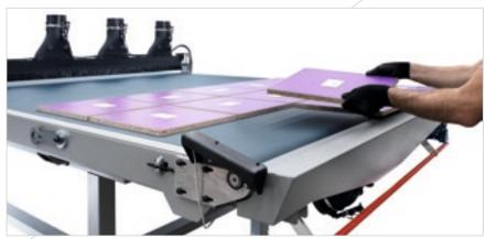
Machine efficiency is dramatically increased due to the **unloading belt**, which enables the removal of completed components outside the machine's work area.
