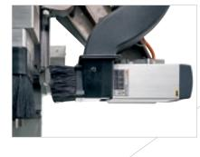
The multi-function unit, which can be continuously positioned over 360° by NC, can house aggregates used to carry out specific machining operations (pocketing for locks, hinge housings, deep horizontal bores, edge trimming, etc.). Horizontal motor with one outlet for lock routing and horizontal machining operations.
