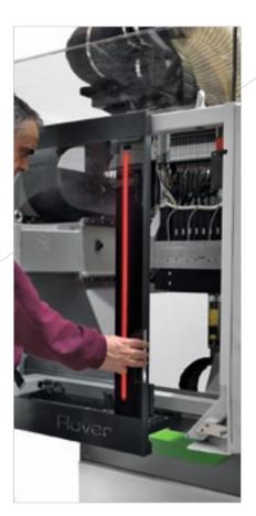
Long term safety and reliability thanks to the new **bumpers** combined with **photocells** with no footprint or mechanical wear.
