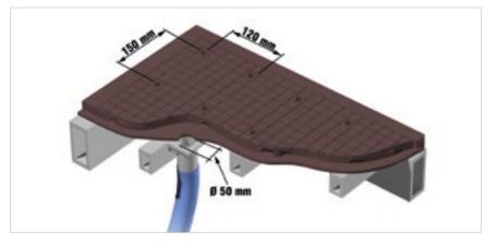
**Multi-zone** technology able to concentrate the vacuum in smaller areas of the work table where required, in order to hold smaller components and reduce vacuum loss.
