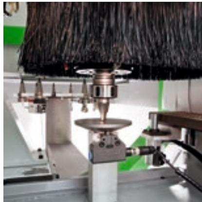
Reduction of tool change set-up time and the possibility of operator error, thanks to the **contact pre-setter**, which automatically determines the length of the tool.
