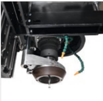
The **loop presser** supports the machining of curved and stacked panels by applying pressure to the upper surface of the panel.
