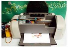
Use the color inkjet printer (with heat transfer ink) to print the picture on the heat transfer paper (setting mirror image printing style)
