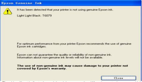
• The chip will not indicate the real-time ink consumption. When it runs to the assumed ink limit, the relative Ink-out area blinks and the panel shows REPLACE INK CRTG. A chip resetter is needed to make the chip reuse.
