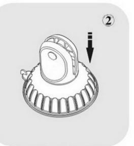
Press it to make the suction cup fixed on the surface.
