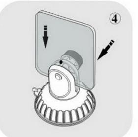
Insert the drilled board into the channel on top, and fix it by screw.
