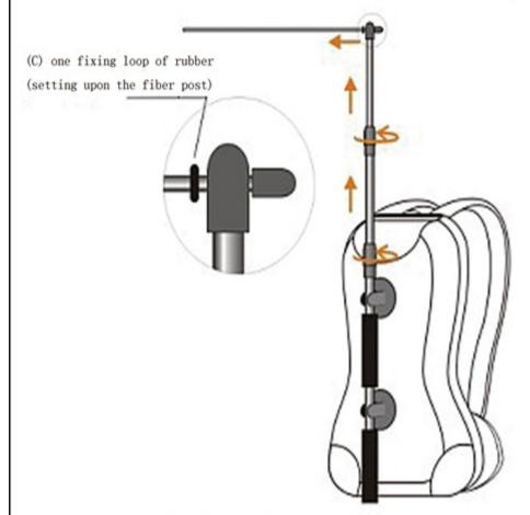
Unscrew the expansion bend to adjust the height of flag pole and thrust the fiber post, then set the fixing loop of rubber.
