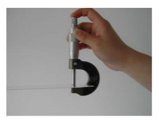
Length tolerance is -2/+0.1" (3mm), width tolerance is -1/+0.1" (2mm), thickness tolerance is  $\pm 0.05$ mm.
