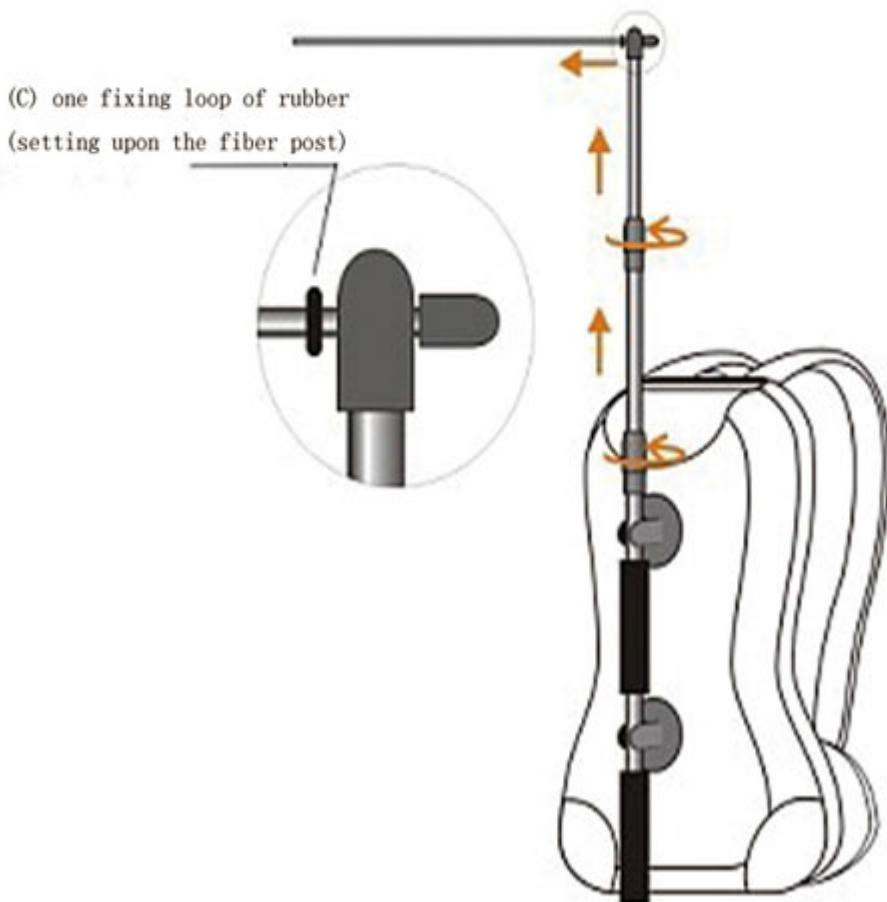
Unscrew the expansion bend to adjust the height of flag pole
