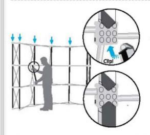
4, Apply the bars to all vertical quadrants on front side of the frame and to each end on back side of the frame. For a double sided frame, apply the bars also on the back side of the frame.
