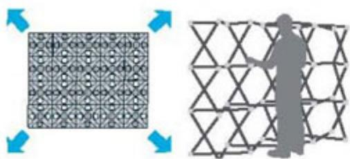
3. Place the frame on the floor with hubs with graphic hangers facing up and towards you. Grasp frame scissors and lift to expand frame
