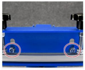
Chuck can adjust the frame height according to the thickness of the substrate
