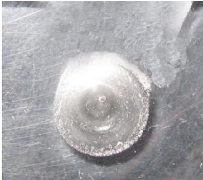
Laser spot with depth of 5mm
