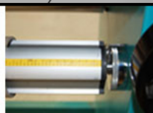
New type aluminium alloy supporting roller
