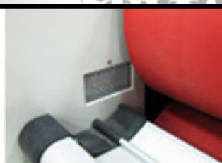
The baffle - board of photocell safety switch
