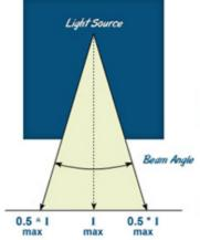
**Beam Angle** is the degree of width that light emits from a light source. In specific terms this is the angle between the opposing points on the beam axis where the intensity drops to 50% of its maximum. We normally produce 60 degree and 120 degree beam angle lights.
