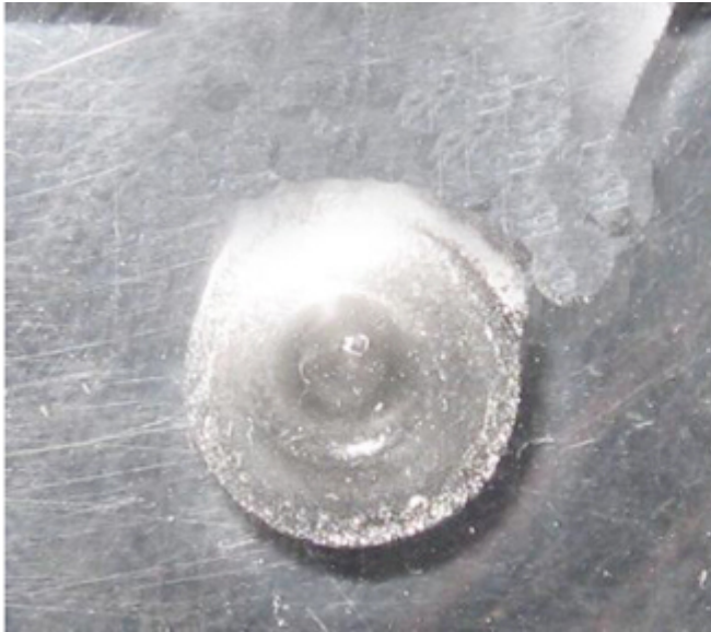
Laser spot with depth of 5mm
