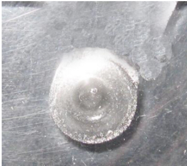
Laser spot with depth of 5mm
