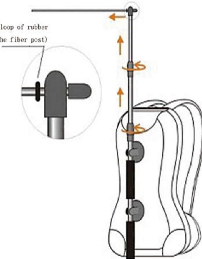
Unscrew the expansion bend to adjust the height of flag pole and thrust the fiber post, then set the fixing loop of rubber.
