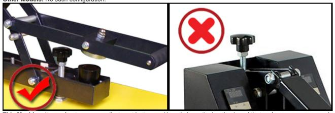
**This Machine:** It uses front pressure adjustment button positioned above the heating board that performs more averaged pressure on. **Other Models:** With rear pressure button that makes unbalanced pressure.
