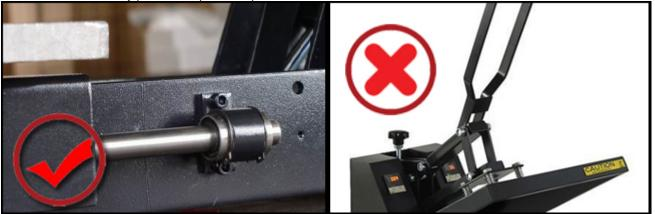
This Machine: It uses sliding bearing with stretchable worktable which increase your work space and very convenient for placing transferring objects.
