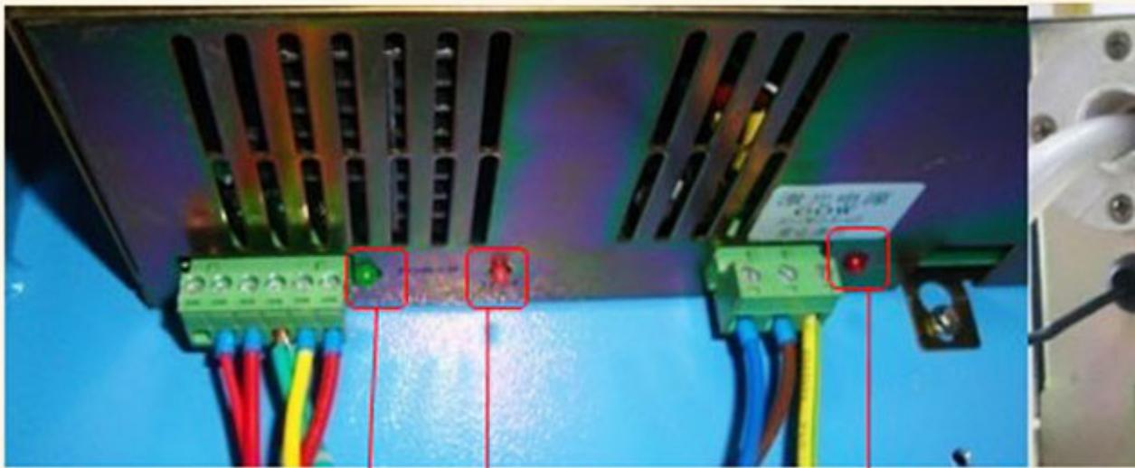
Power indicator lamp Test button Laser indicator lamp
