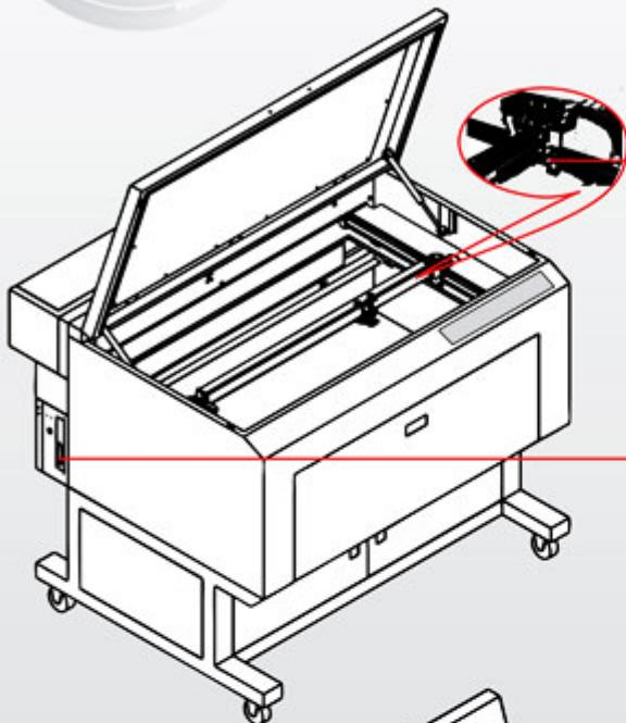
5. Remove the X axis locking screw
