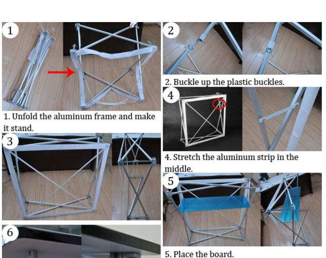
6. Install the top board onto the frame by plugging buckles to relative holes.
