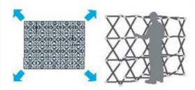
3, Place the frame on the floor with hubs with graphic hangers facing up and towards you. Grasp frame scissors and lift to expand frame
