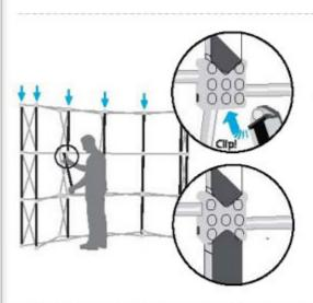
4. Apply the bars to all vertical quadrants on front side of the frame and to each end on back side of the frame. For a double sided frame, apply the bars also on the back side of the frame.
