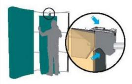
Hang the graphic panels on the top hub-hangers letting panels attach to bars. Do the same on both end-caps of the frame.
