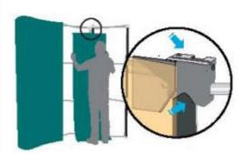
5, Hang the graphic panels on the top hub-hangers letting panels attach to bars. Do the same on both end-caps of the frame.
