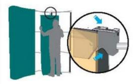
Hang the graphic panels on the top hub-hangers letting panels attach to bars. Do the same on both end-caps of the frame.
